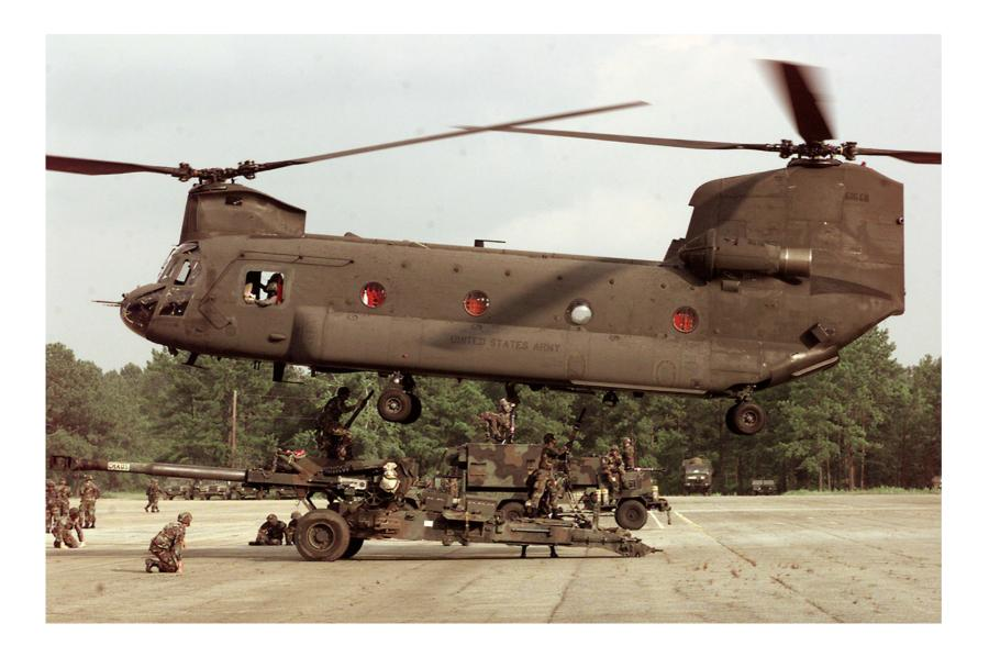
A U.S. Army CH-47 Chinook. First introduced in 1962, this American twin-engine, tandem rotor heavylift helicopter was primarily used for troop movement, artillery placement and battlefield resupply.
