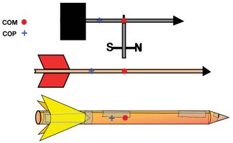
The positions of center of mass (red dot) and center of pressure (blue +) are shown for a weather vane, arrow, and rocket. The center of pressure is to the rear of the center of mass in each device. This enables them to point into the wind.
